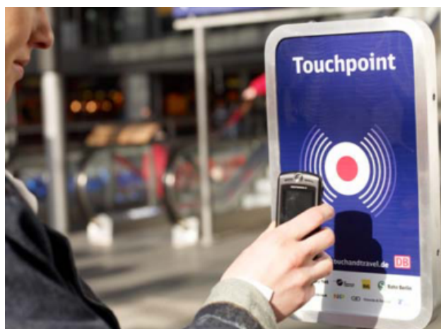
Figure 2.2: Touch & Travel Near-Field Communication (NFC) smartphone validation system used in DB Bahn [Gem08]
